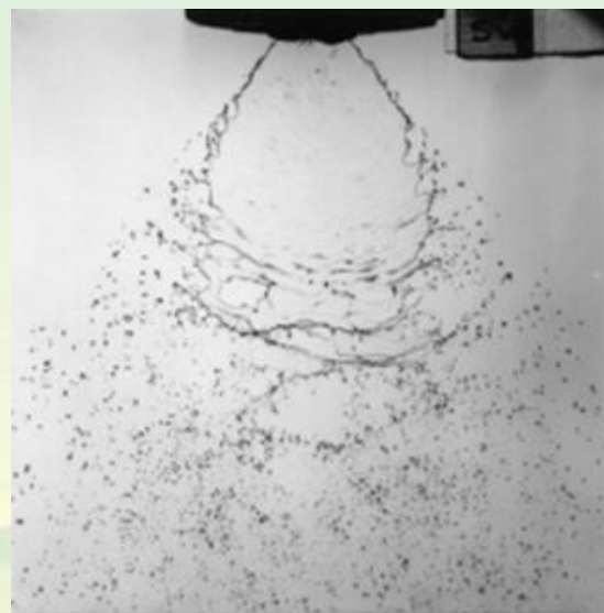
Standard flat fan nozzle spraying Water at 1.0 bar
